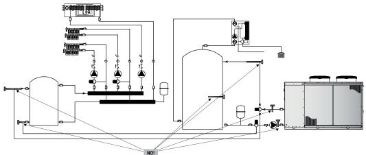
4.24 Positioning of the domestic hot water circuit sensor (BTS)
