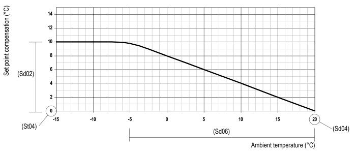
All units are factory set with the weather compensated function activated. The slope starts at +20°C with a differential of 10°C.
