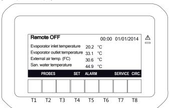
When the digital input is not active, the unit is in OFF mode
