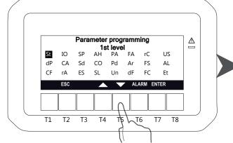
Setup parameters (SP): make possible to modify the serial address.
