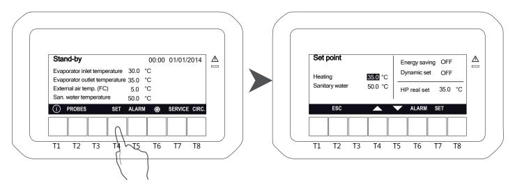
To modify the values, move the cursor with rescaled, press SET to select, the value starts blinking, change the data pressing and . Once the required value is reached, press again SET to confirm.
