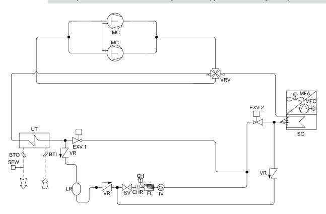
Models LHA 2504 - 3004 - 3204 - 3504, 4004 - 4504 - 5004, in all versions, use two independent refrigerant circuits identical to the one shown above.
