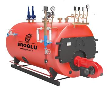
**EROĞLU SBK** Series, are fire – smoke tube 3- pass high pressure boilers between 0.5-20 bar pressure and 0.5-15 ton /h. it is the most frequently used scotch type boilers. SBK steam boilers are manufacture and guaranteed by the over thirty years of experience of **EROĞLU** in the construction of industrial and professional boilers which are installed and appreciated all over the world. SBK series steam boiler design to produce: saturated steam, superheated steam, low pressure steam.
