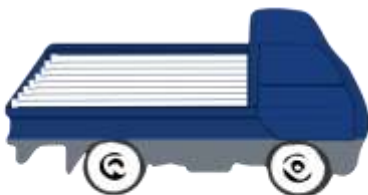
correct way to load pipes
