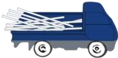
Incorrect way to load pipes
