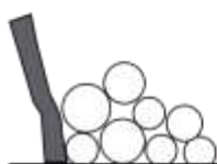
Incorrect way to stack pipes
