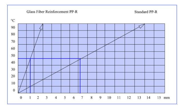
While glass fiber reinforced PPR pipe elongates 1.75mm in 1 meter at temperature difference of at 50°C, on the other hand standard PPR pipe elongates 7.5mm in 1 meter in the same temperate difference
